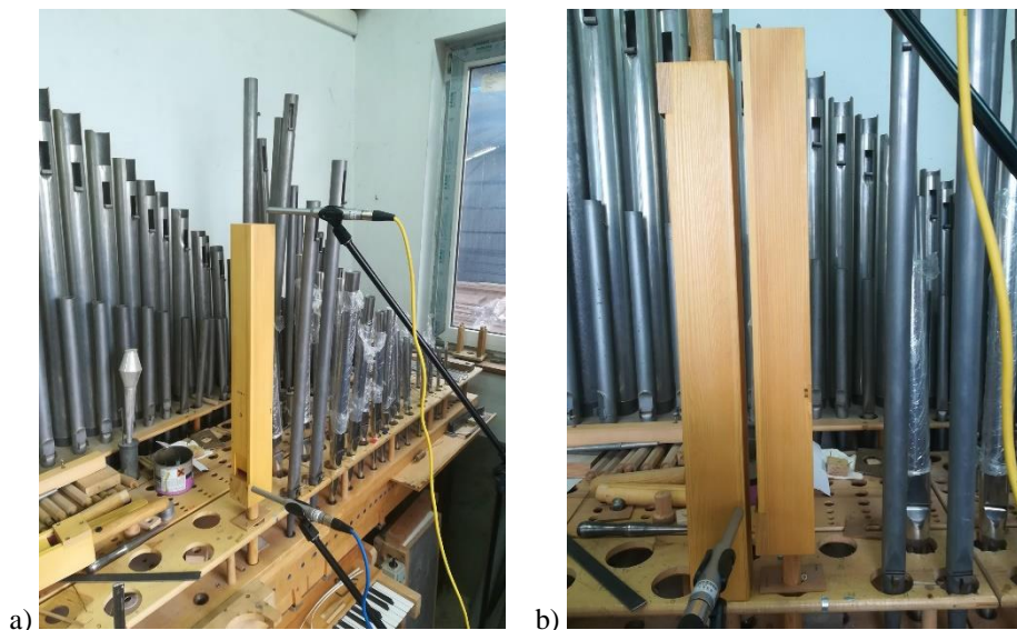
Figure 1. Measuring point and sample measurement for Bourdon 8-foot: a) without obstacles, and b) with an obstacle
