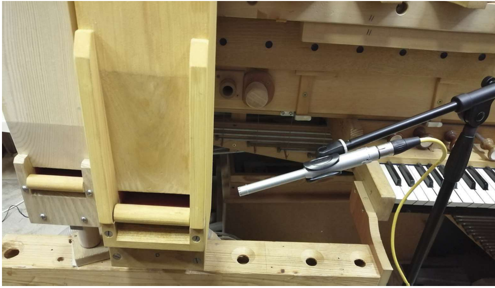
Fig. 2. Microphone setting in the process of pipe sound recording.
