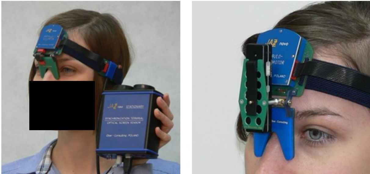
Figure 3. Studies [A3], [A4] used a head-mounted saccadometer JAZZ (Ober Consulting, Poland), which was able to measure the reflexive saccades (RS) in the high frequency (1000 Hz). The advantage of this setup is lack of disruption from head movements.
