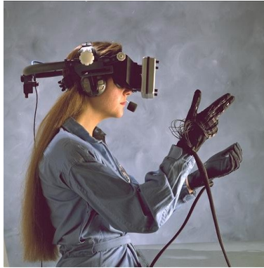
Fig. 3. VR Goggles developed by NASA's Ames Research Center in 1985, and wired gloves.
