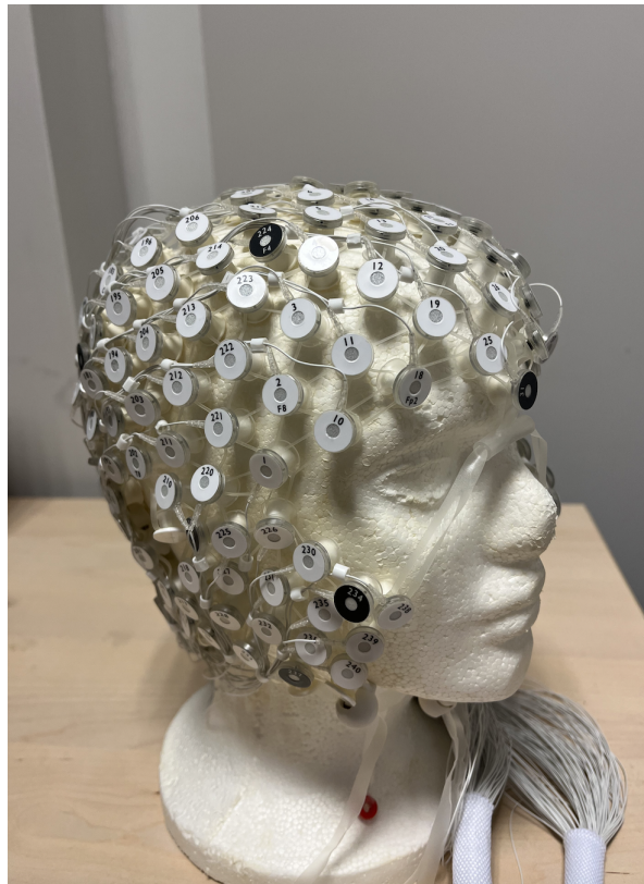
Figure 4.5: Cap for measuring the EEG signal from the surface of the scalp
