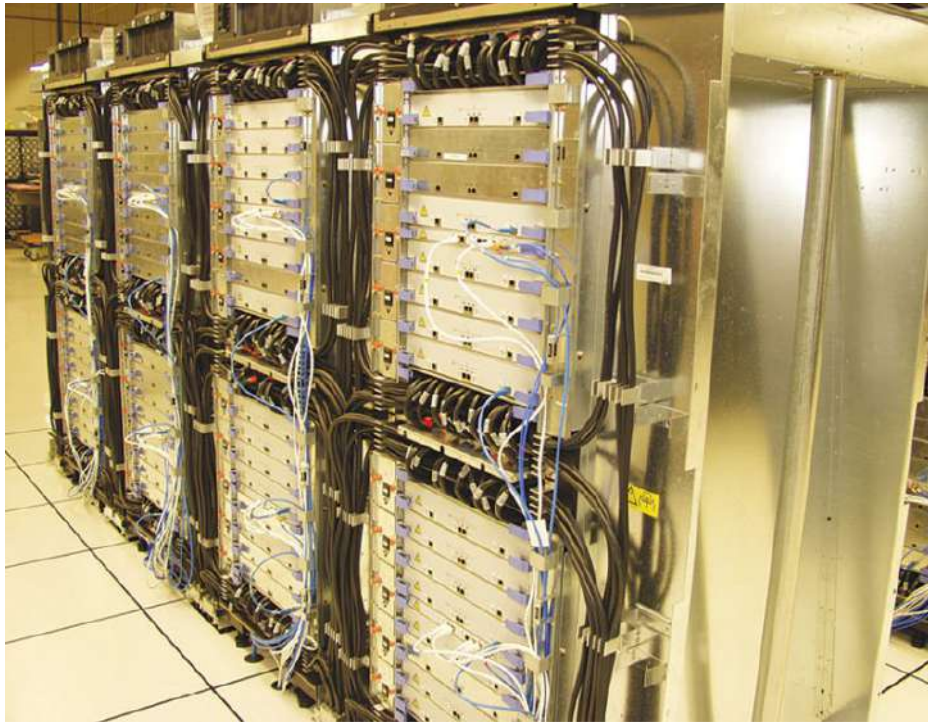
(a) IBM BlueGene/L supercomputer used in the early stages of the Blue Brain Project.
