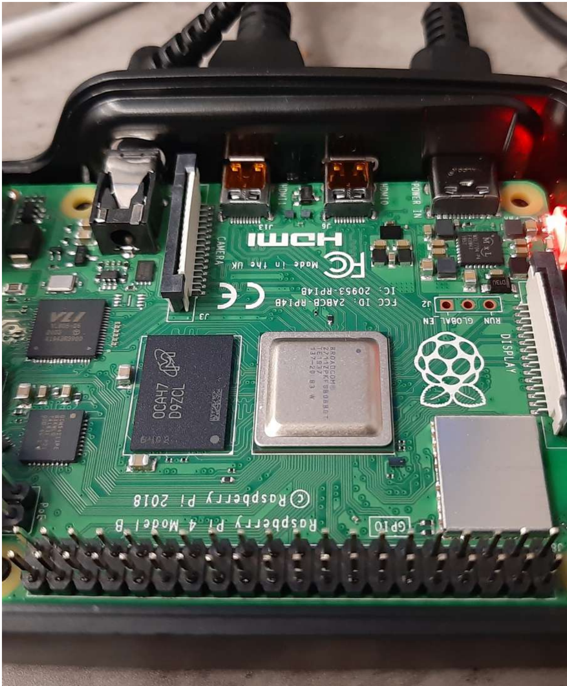
Fig. 3.5 Author's Raspberry Pi 4 Model B single-board computer that was used in simulations, and as part of Neural Simulation Cluster.
